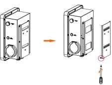
STEP 2: Fix the back bracket and the cable hook (only for type P) to the wall.
