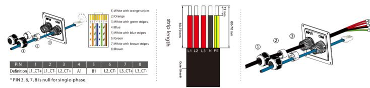
STEP 9: Insert the wires into the appropriate holes of the terminal blocks, then block the terminals with the straight screwdriver.
